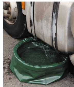
A small portable container in use to contain a fuel leak.
