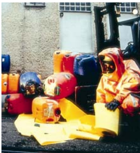
Chemical sorbent being used to contain a small spill.
